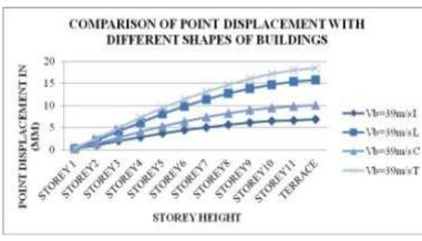
Fig. 7. Variation of Lateral Displacements with height
